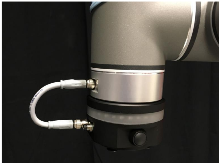
Figure 5 Physical mounting of the YOuring.
