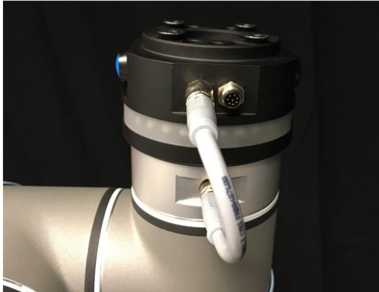
Figure 4 Physical mounting of the YOuring.
