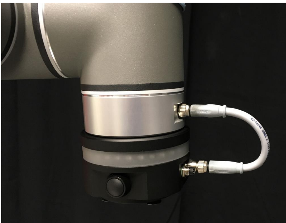
Figure 13 View of the freedrive button
