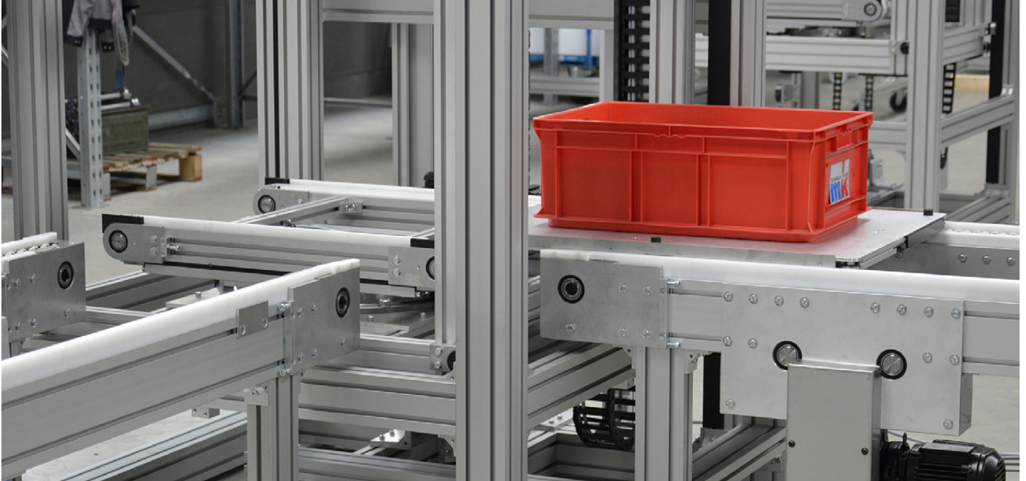
Different modules can be combined to make a single unique module, such as the right angle transfer unit, mounted within a Vertical Transfer Unit.
