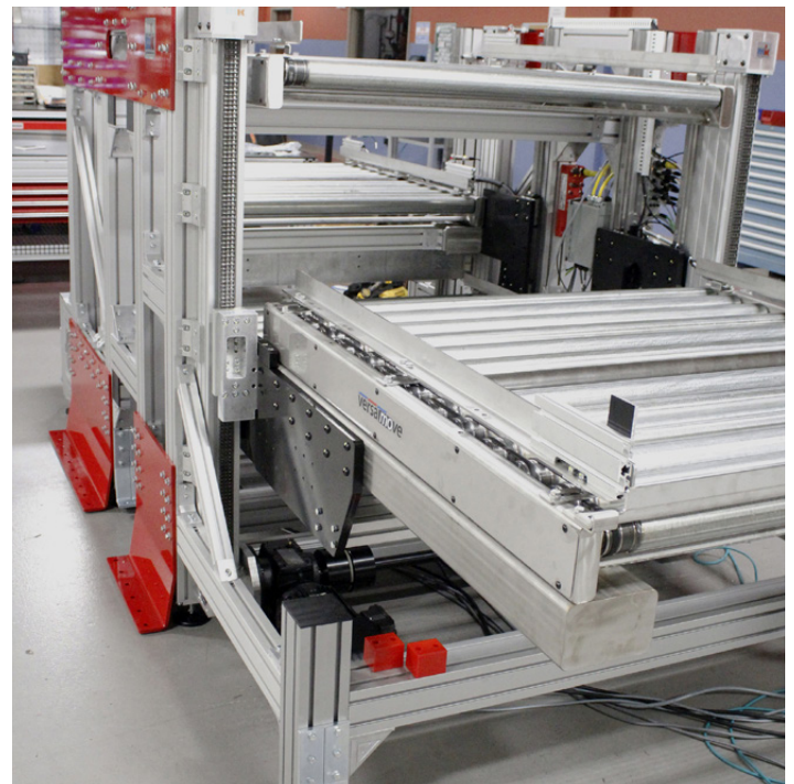
mk is able to accommodate customizations including custom transfers such as custom vertical transfer units featuring roller conveyors.
