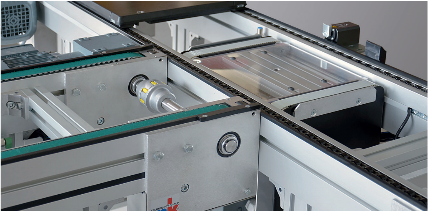
HQZ 2045 Lift and Transfer designed to transfer a pallet from a ZRF-P 2045 Timing Belt Conveyor to a SRF-P 2045 Accumulating Roller Chain unit.
