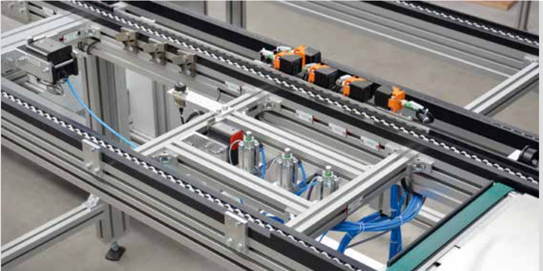
Versamove plus: Customer-specific special stopper unit with four removal positions
