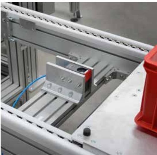
Versamove ultra: Accumulating roller conveyor with special chain guides for higher loading
